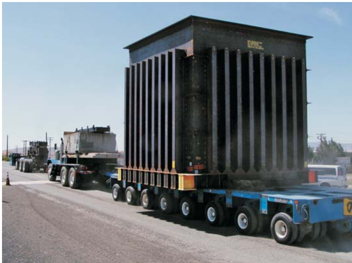
To meet transportation requirements, this custom steel box was delivered to Hanford for shipping the tanks.
