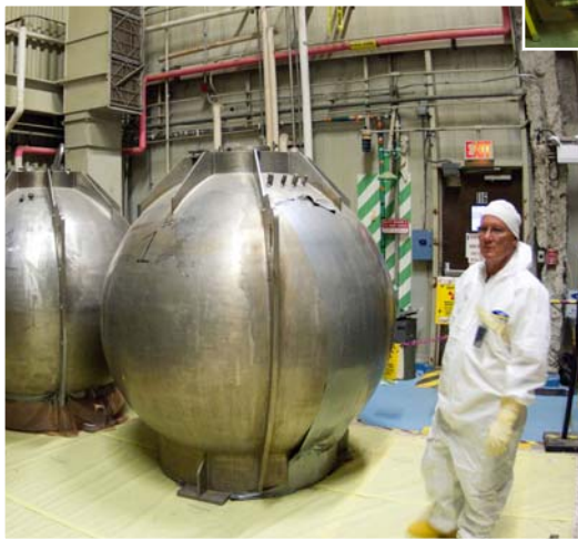
Lead-shielded 60,000 pound casks delivered high-level radioactive materials to 324 for research.
