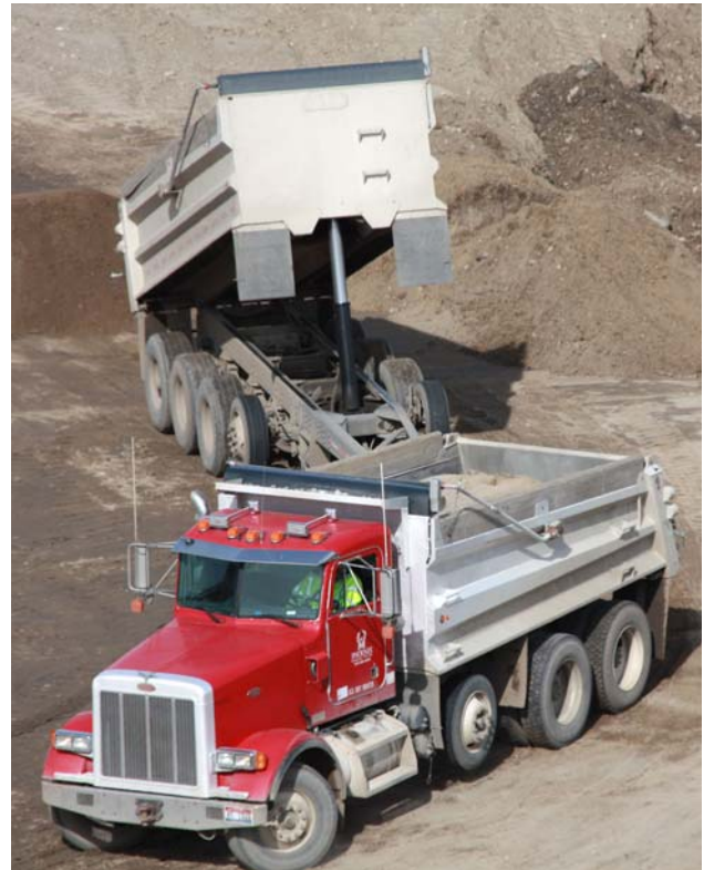
Washington Closure Hanford began using truck and pups in July 2009 to transport non-regulated, non-radiological waste to ERDF. The operation has helped the Waste Operations team to safely and efficiently meet disposal demands.
