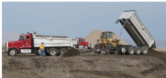
A truck and pup can hold 30 tons of material, about one-third more than a roll-on/roll-off waste container.
