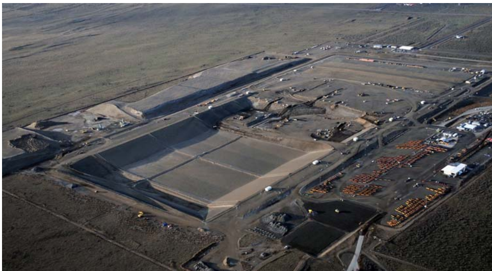
Super cells 9 and 10, in foreground, cover an area of 33.6 acres and have a capacity of 5.6 million tons.
