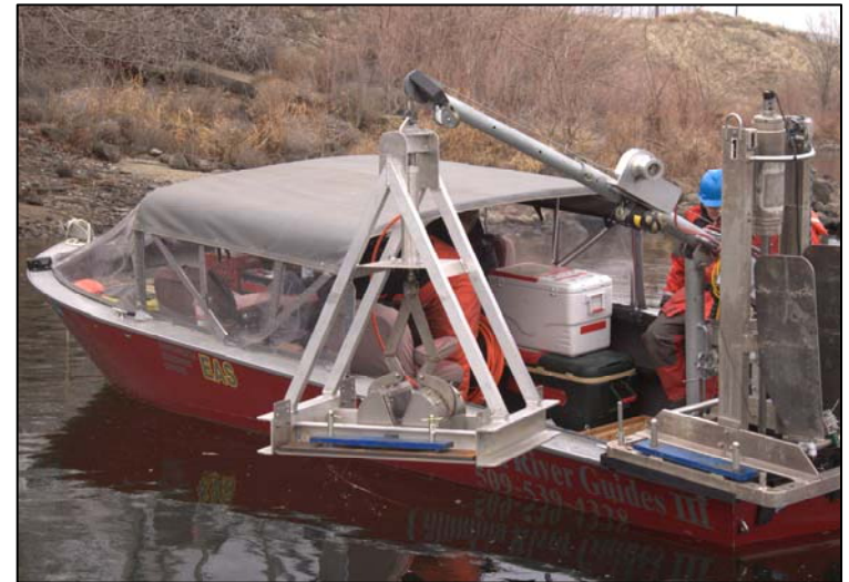
Deployment of Power-Grab Sediment Sampler Unit in Support of Columbia River Remedial Investigation
