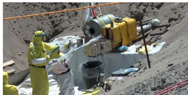
Soil samples directly below B-Cell were retrieved in June 2011. Lab analysis will provide key information for selecting cleanup options.
