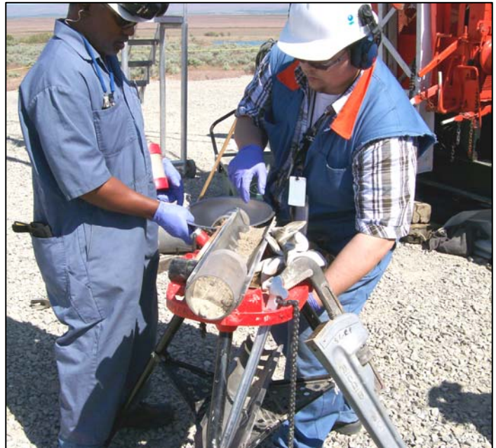
Collecting Soil from Split-Spoon Sampler at 100-K Area
