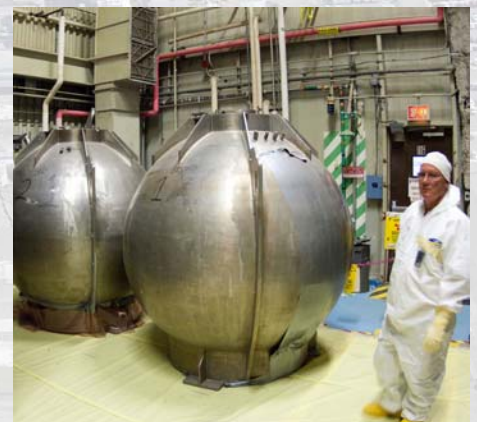
Dave Jenkins next to lead-shielded 60,000 pound casks used to deliver high-level radioactive material to 324 for experiments in hot cells.
