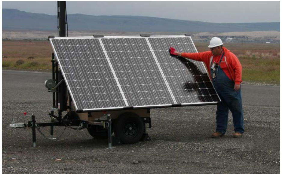
Royal Shuler, stationary operating engineer at the 100-N Area Waste Pad, wipes down the collectors on the solar-powered lighting plant, which was part of a pilot-project conducted at the intersection to N Area last spring.
