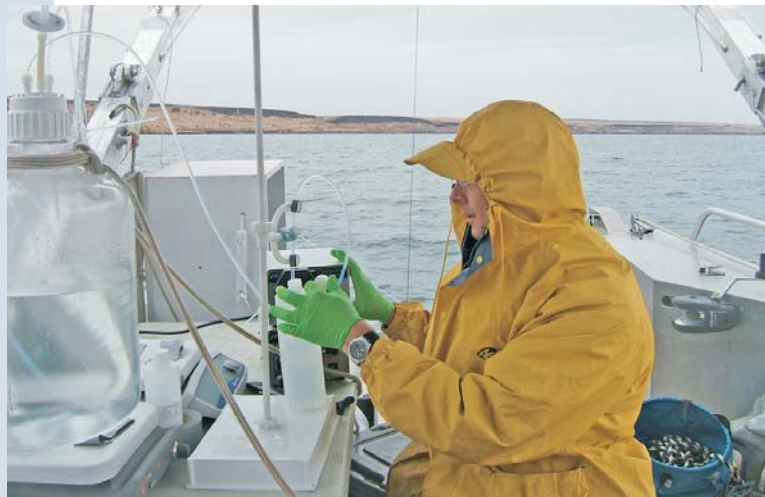
Water sampling includes groundwater upwelling into the Columbia River. This investigation will help identify sources of contamination for final cleanup decisions.
