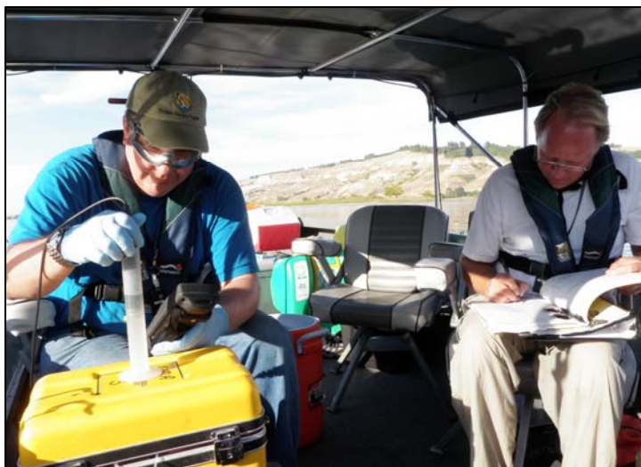
Collection of Pore Water Samples Using the Trident Probe Technology
