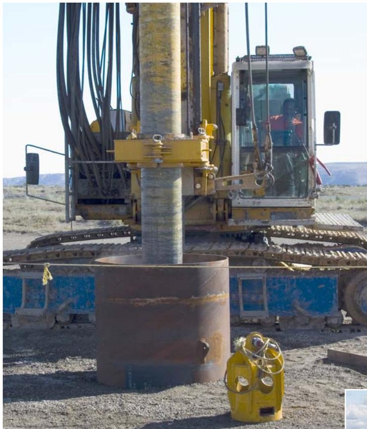
Material in a simulated drum style VPU is augered during method testing.
